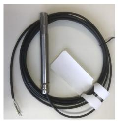
Digital humidity / temperature sensor based on electrolytic-resistive measurement technology. In stainless steel body and 5 meter bus cable.
